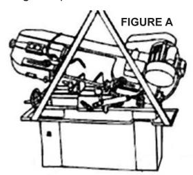
4. Once the Bandsaw is lifted, insert the Wheel Rod (92-4) through the two holes located at the bottom/right side of the Stand (77S). Slide one Wheel (92-2) on each end of the Wheel Rod. Place one Washer (92-1) on each end of the Wheel
